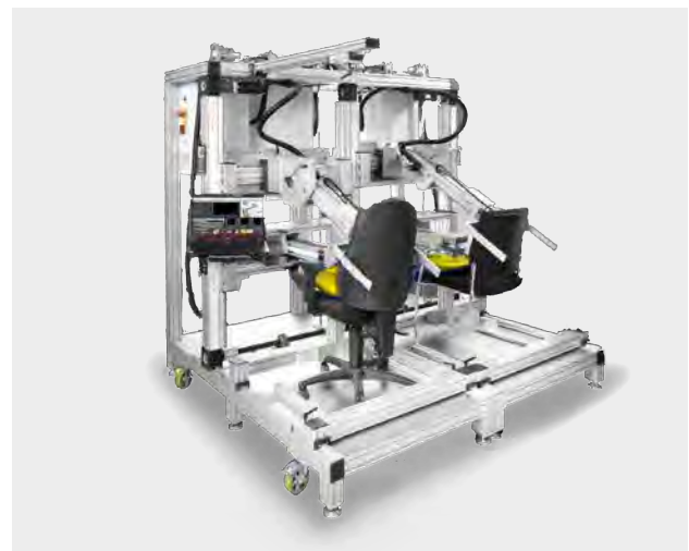
Bending change test stand with servo axes
